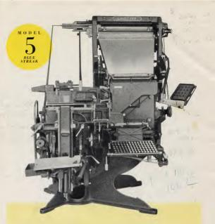
INTENDED for composing rooms that require a single-magazine Linotype. The standard 90channel magazine is quickly and easily removed from the foruk using the same convenient Inbuilt Magazine Change Mechanism which is found on all Blue Streak Linotypes.
